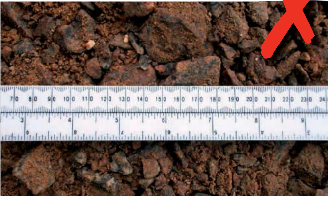
Type 1 aggregate for conventional block paving is not permeable when compacted.
