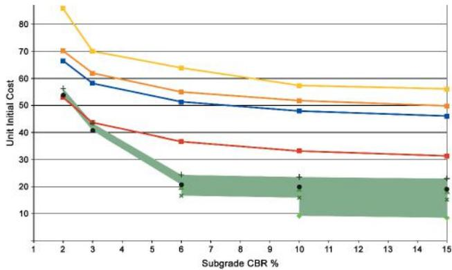
The loading regime on an industrial estate distribution road can be relatively severe, with a high proportion of heavy good vehicles. So, maintenance and WLCs are important, with CBPP (System C) offering the lowest WLC.
