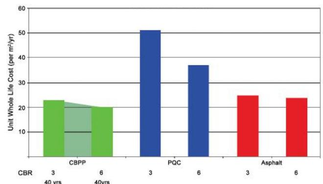
**Estate Roads – Industrial** – Initial costs for all types of CBPP are substantially lower than asphalt for CBR values of 4% or more, becoming similar for the lower values.
