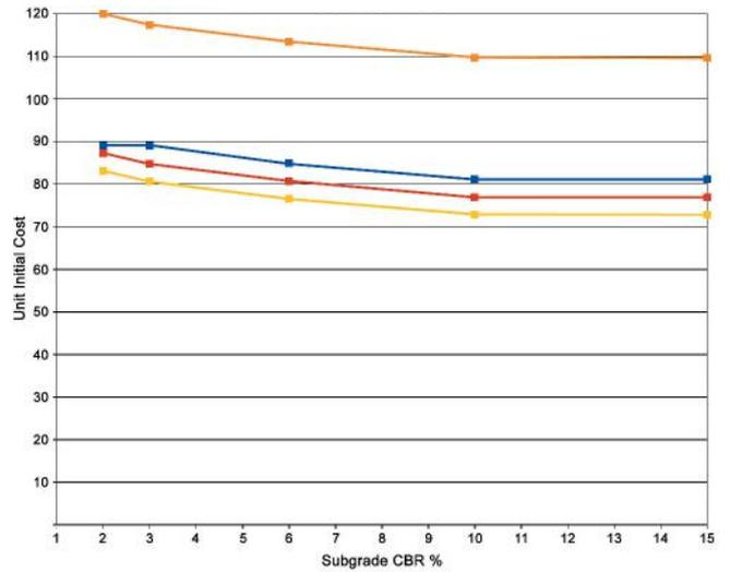
**Airport Airside Pavements** – considered from an initial cost perspective only. Costs of impermeable concrete block paving follow those for asphalt and are substantially lower than those for reinforced or PQ concrete until very low CBR values are reached.
