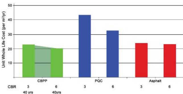
**Container Yards** – considered from an initial cost perspective only. Costs of impermeable concrete block paving are slightly lower than both asphalt and PQ concrete for all CBR values with reinforced concrete substantially higher.
