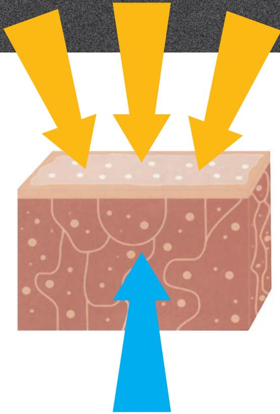
**Efflorescence emerged from pores within a magnified area of a concrete paver. The calcium has been carried to the surface by water.**
